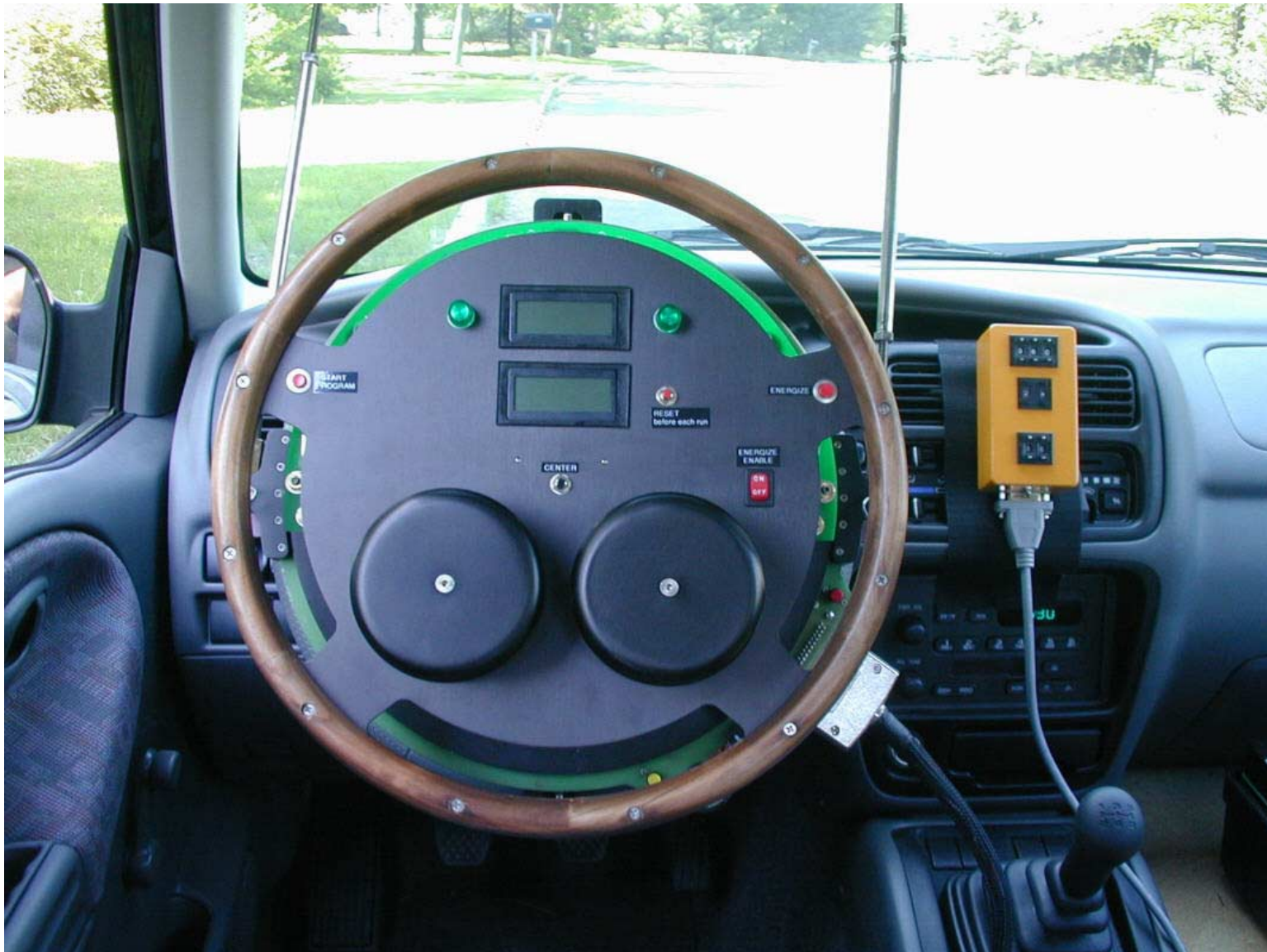
Figure 2: Sprint 3 machine and Command Module installed in vehicle.
