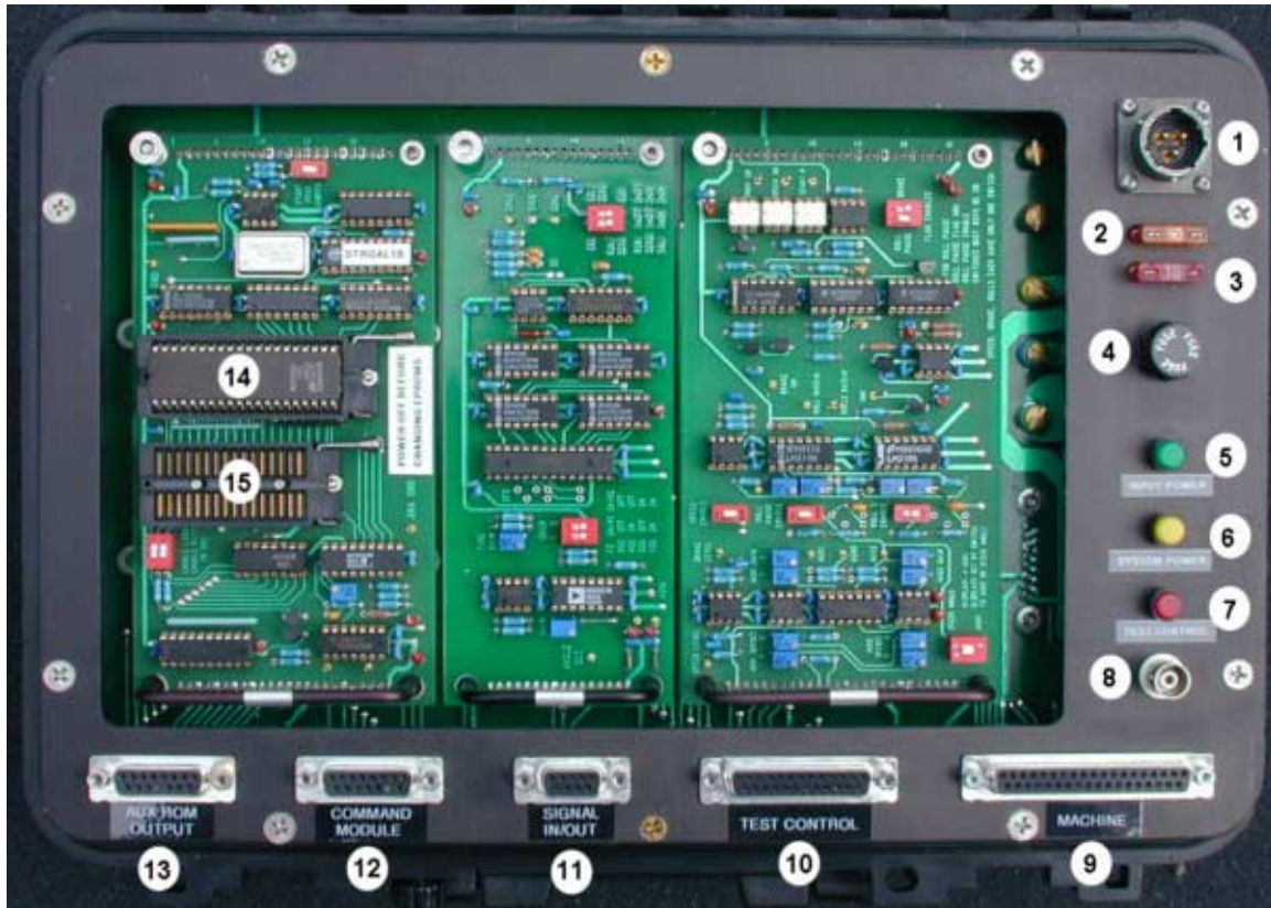
Figure 3: Sprint 3 Steering Machine Electronics Box Connections
