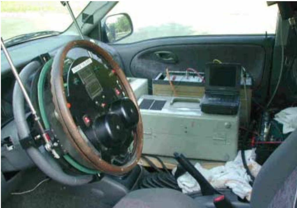
Figure 4: Steering Machine in foreground; Stable Platform with VTR atop (center), Data Acquisition system (rear) in background.
