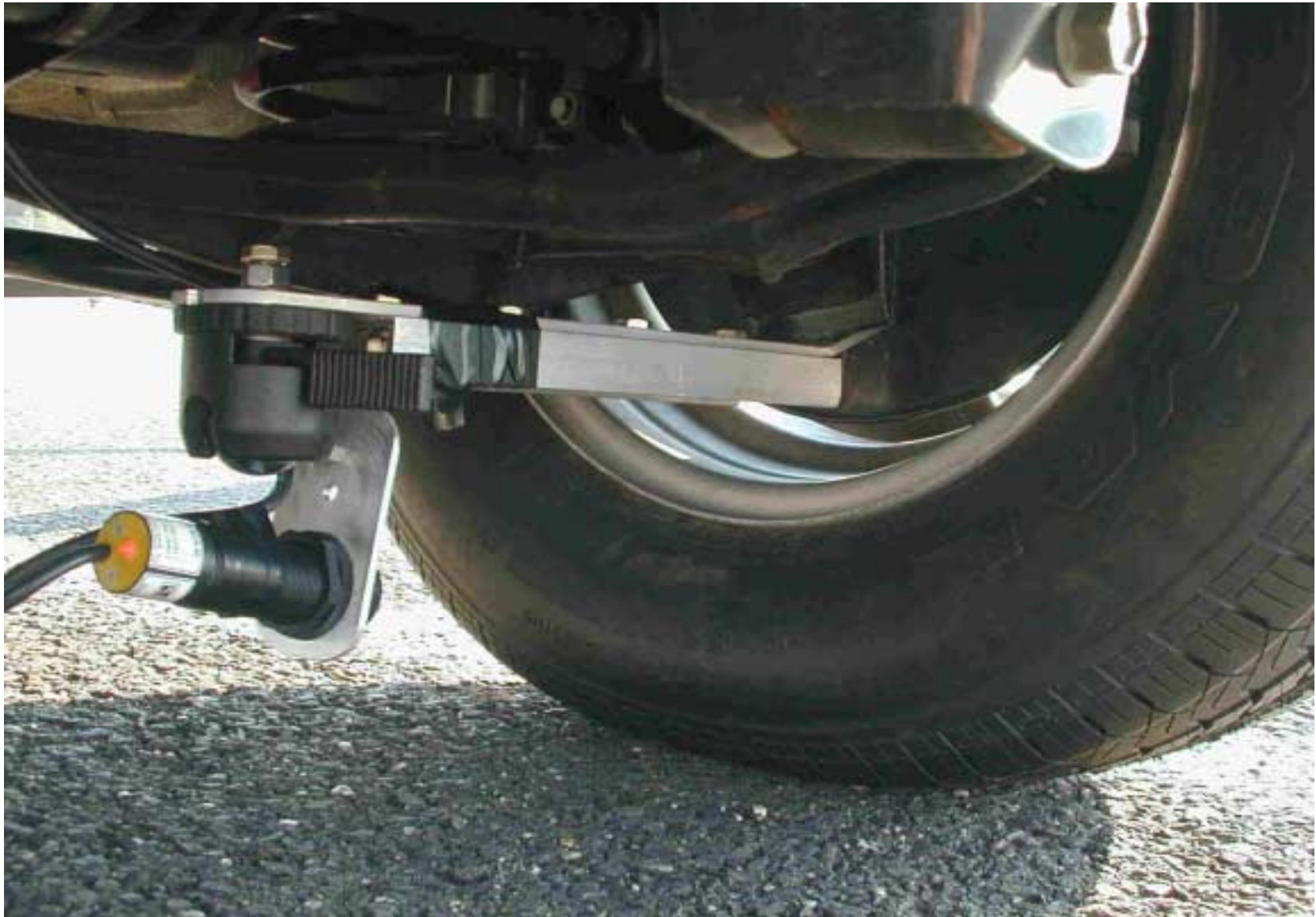
Figure 5: Ultrasonic transducer for tire lateral deflection.
