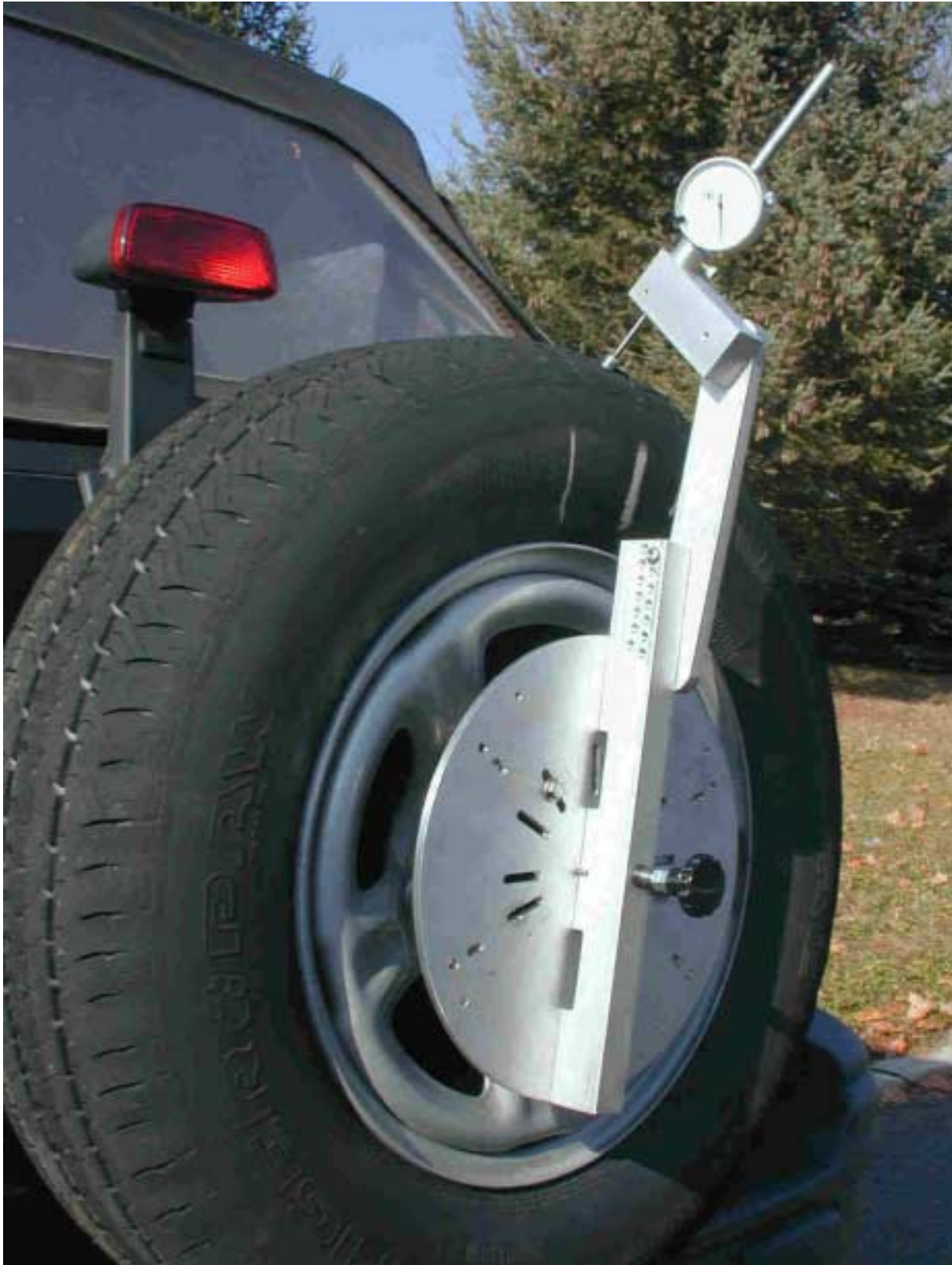
Figure 6: Tire shoulder wear measuring assembly (Right front tire after test).
