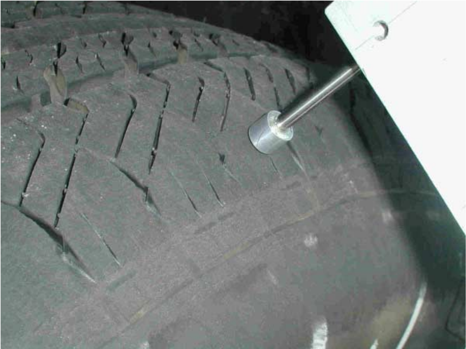
Figure 7: Right front tire with dial indicator after Run #18.
